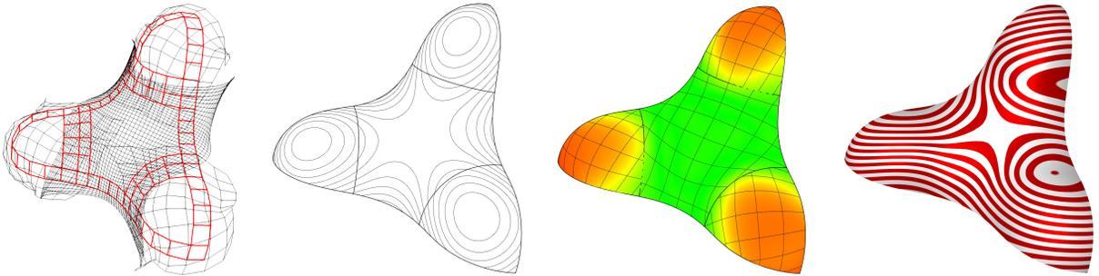
Fig. 4: A model with four trimmed patches shown with contours, mean curvature and isophote lines.
