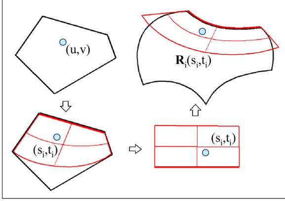
Figure 2: Evaluation of a transfinite surface: (i) point in the polygonal domain (ii) mapping into the domain of each bi-parametric ribbon (iii) evaluating each ribbon (iv) blending the evaluated points
