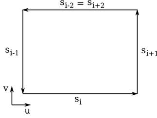
Figure 1: Domain of a Coons patch using side-based parameterization
