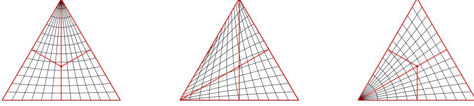
Figure 6: Control nets for triangular domains, based on the bottom side (left image), the right side (right image) and both (middle image).
