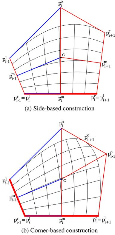
Figure 5: Control net and constant parameter lines of the bi-quadratic parameterization.
