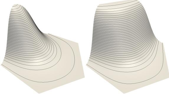
Figure 3: Blending functions  $B_{i,i-1}$  and  $B_i$  over a six-sided domain.
