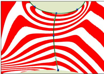
Figure 11: A  $G^1$  model with two composite ribbon patches, using isophote line visualization.
