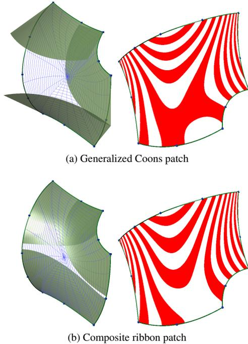
Figure 10: Ribbons and slicing map of a five-sided boundary configuration.
