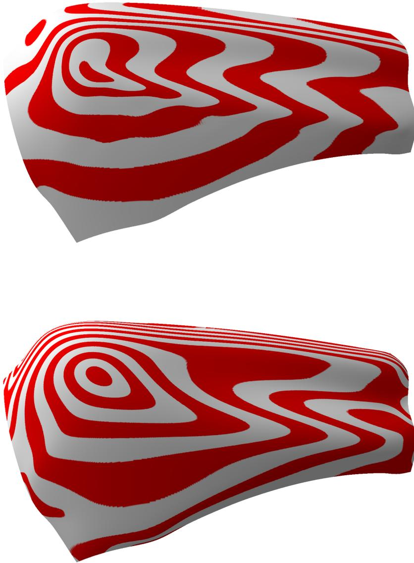
Figure 2.6: Surface fairing by PDE-based extension of the target curvature algorithm.
